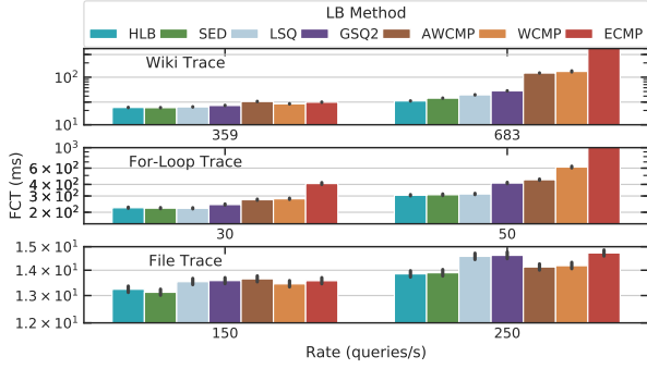
Figure 21. [Testbed] Comparison with different types of network applications.
